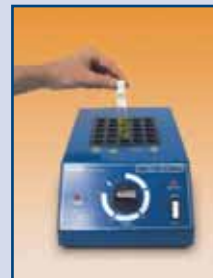
2. Place the vial in the HI 839800 reactor (sold separately) and set the timer
