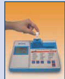
3. Place the vial in the HANNA HI 83099 and read the results
